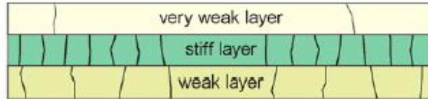
Spacing of bedding-parallel joints according to competence (elastic modulus) of layers
